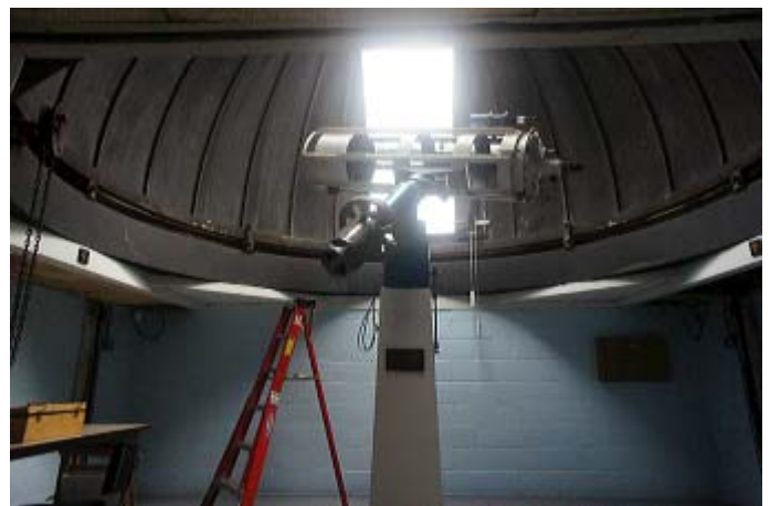
The second veteran scope (and first MVO scope) is the Draper-Prather 16" Cassegrain. It sat in its newly painted building. This was the "big scope" for many years. Always proving that bright images at high magnification is the way to go.
